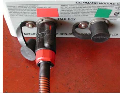
10. Connect the other end of the cable to the “Talk Box”. These connections are labeled in blue.
