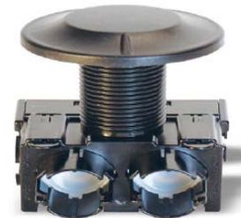
Sensus leak detection technology is the Permalog+ which uses sound waves to monitor distribution lines and localize leaks. Sensors activate overnight, listening to the distribution system when ambient noise is at its lowest, then report pipeline conditions back to the utility via FlexNet.
