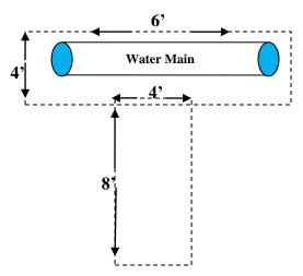
After traffic control and excavation are ready please notify the Water Division Lead Operator and Public Works Inspector who assigned to the project. Call for inspection at least 24 hours before tap is scheduled, so that the trench can be inspected and given approval. (See **Public Works Inspection** Step 2 below)
