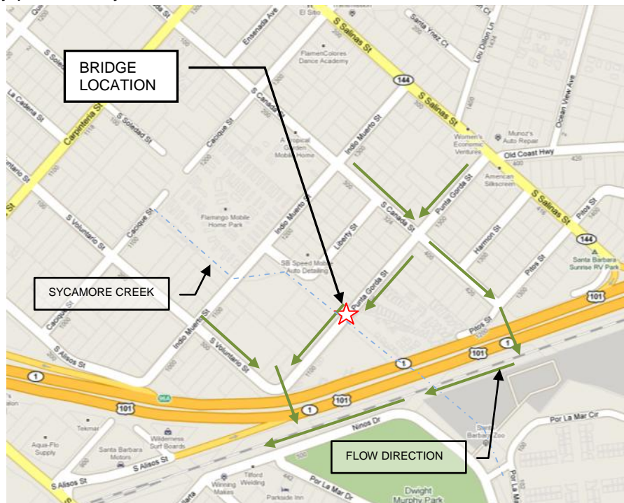
Figure B - Existing Wastewater Flow Patterns
