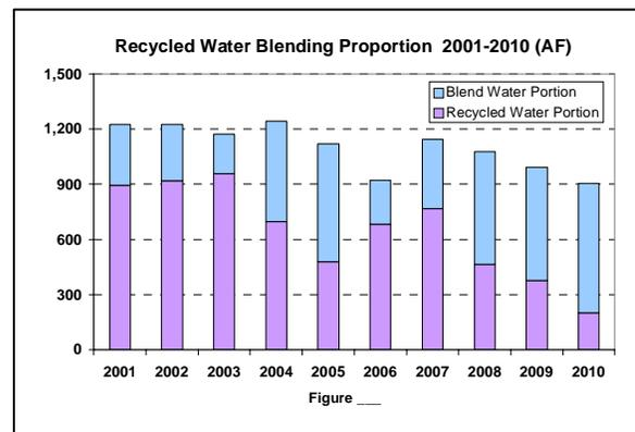
*Secondary Process Issues:* Beginning in 2004, due to challenges with the secondary treatment process, blending has increased recently to approximately 700 AFY to meet regulatory requirements. Improvements to the secondary process are being evaluated to address this recent increased use of potable water for blending. Once the secondary process is resolved, it is expected that the blend water component can be reduced.
