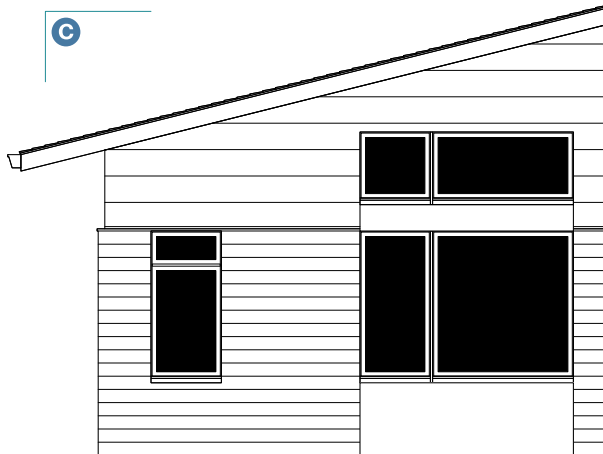
Shed Roof Elevation
