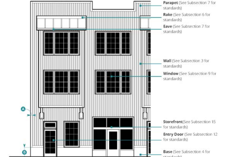
Example Building Elevation: Industrial
